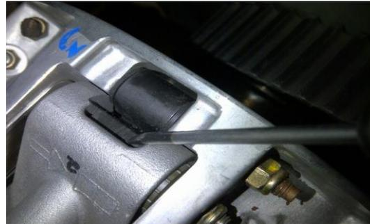
With the moveable sheave / spider assembly back together, keep it together and re-install as a unit, along with the stock primary spring. Install the primary spring into the clutch first, then install the whole unit and **\*torque to spec.**
