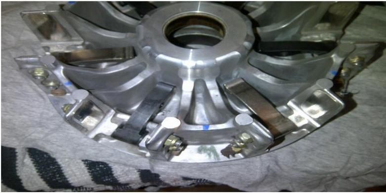
The 3 stock and 3 adjustable weights are alternating. The 3 stock are 120 degrees apart, as are the 3 new ones. – Every second one is replaced. THIS IS THE ONLY CONFIGURATION THAT 3 WEIGHTS CAN BE REPLACED.
