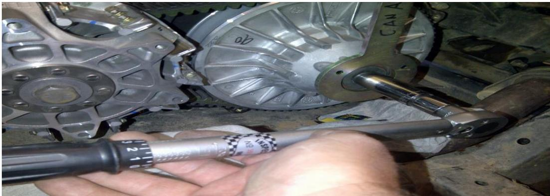
**Torque the secondary ONLY by the BRP recommended procedure !**
