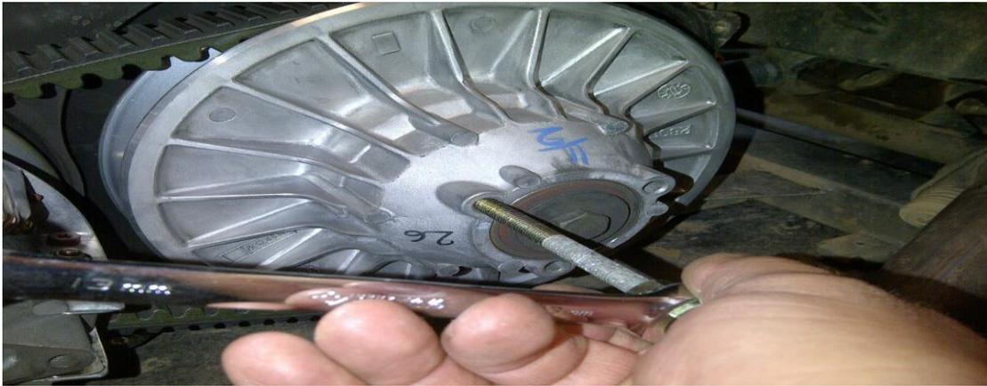
Using the Clutch spreader bolt from BRP (A fully threaded M8 X 1.25 bolt can be used ) spread the secondary make slack to remove the belt.
