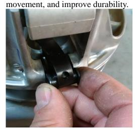
With stock clutches it is common to see the side of the clutch wearing from the flyweight pivot end gouging into the aluminum, even with only low miles. These thrust washers offer smooth function and prevent further wear.
