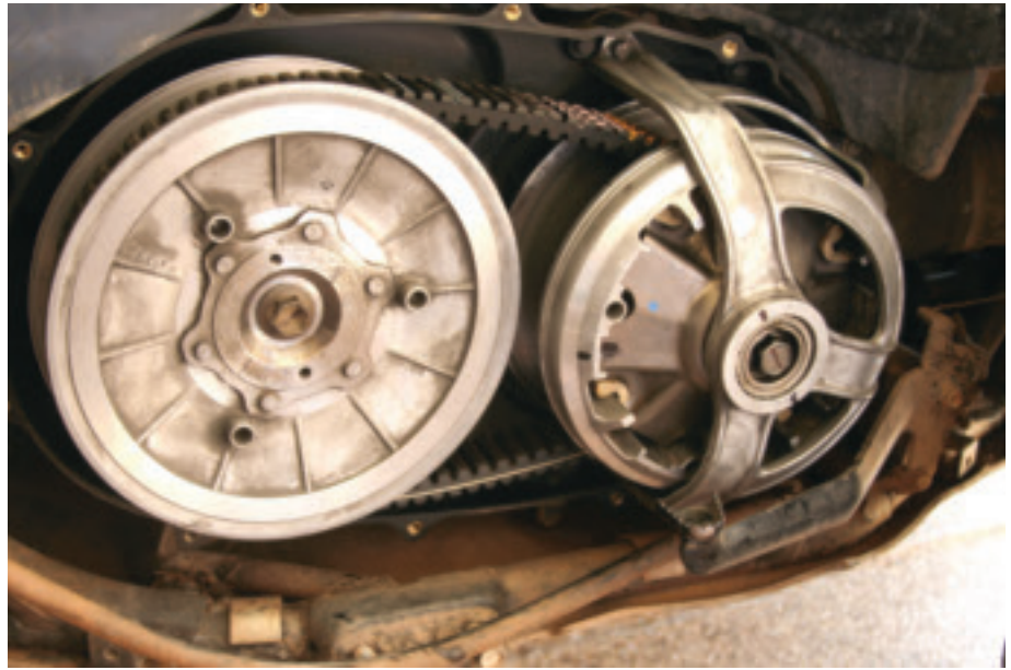
Dalton clutch kit installation complete except for clutch cover and foot rest.
