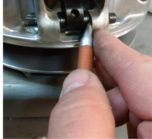
6) Install the new primary spring into the clutch and re-install the cover onto the drive clutch (primary motor clutch). **Note: alignment marks.**
