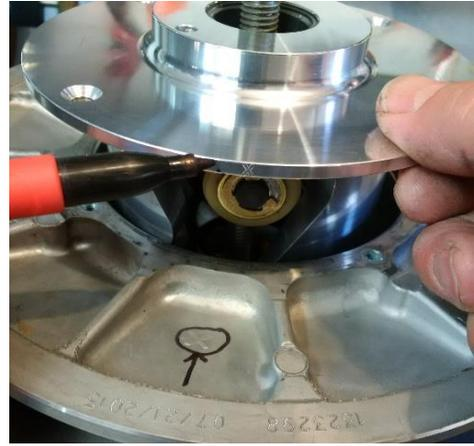
13) Install the T25 screws to hold the helix using a drop of blue thread locker. (48 in./lbs.)
