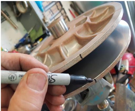
Mark the clutch and take note of both halves and the helix...and position of the roller in the helix for re-assembly. Often, it is best to heat the 3 bolts slightly to release the thread locker before removing.
