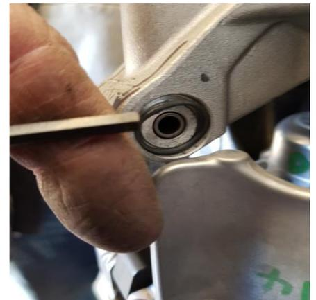
**Change primary spring.** Using the threaded compressor tool, close the tool down onto the spring retainer cap to contain the spring while the screws are removed. Do not over tighten the tool onto the retainer.
