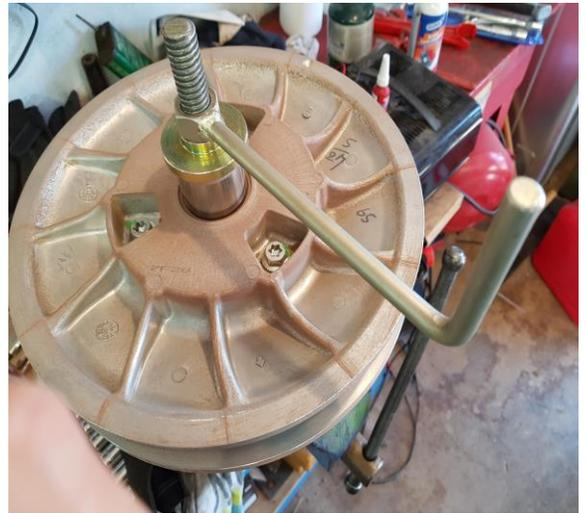
When you assemble the new helix and spring, the helix and pulleys that must be aligned. It is important to have the **“roller” of the clutch in the proper slot of the helix and the torsion spring set correctly.**
