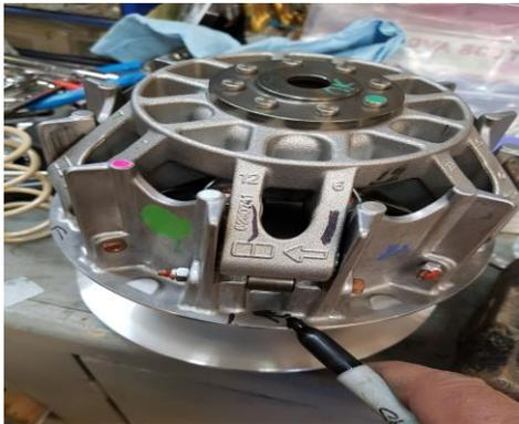
It is **important** that the **o-rings** get put in place properly so that the governor assembly will slide down into the slots correctly. If o rings are not in the groove it will damage the o-rings and the clutch will not slide correctly. It is normal to be slightly stiff sliding, but if it is tight the o-rings may not be in place correctly.
