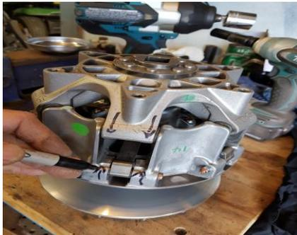
Remove the governor cup puller tool from the drive clutch
