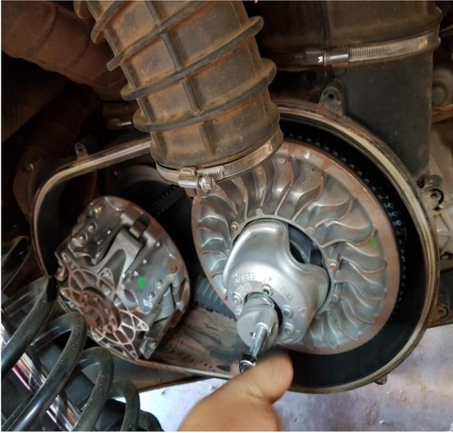
Figure 1- spread secondary(rear) pulley
