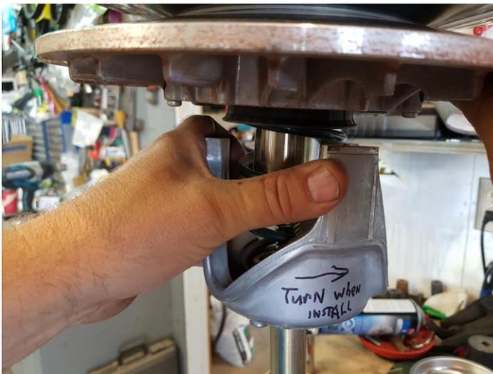
It is very important to make sure the shaft is through the helix bushing before compressing the tool all the way. With the compressor tool installed, it is best to partially compress by hand first and **make certain that the shaft is started through the helix bushing** before using the tool to compress all the way.
