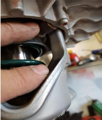
The helix will need to be twisted the proper direction to get the roller in the correct position. The new spring tang will be installed in the same #4 **position on the helix**, but the spring itself is slightly different torsion value and compressed load. The helix and spring must be turned to that same position when you re-install the helix with the new supplied secondary spring.
