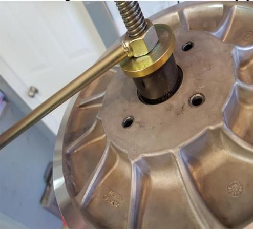
Compressor tool for helix bolt removal
