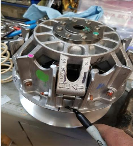
10) **Install Governor /spider assembly back into the sliding sheave.** Make sure that you install in the correct position indicated by the marker **marks** you made previously.
