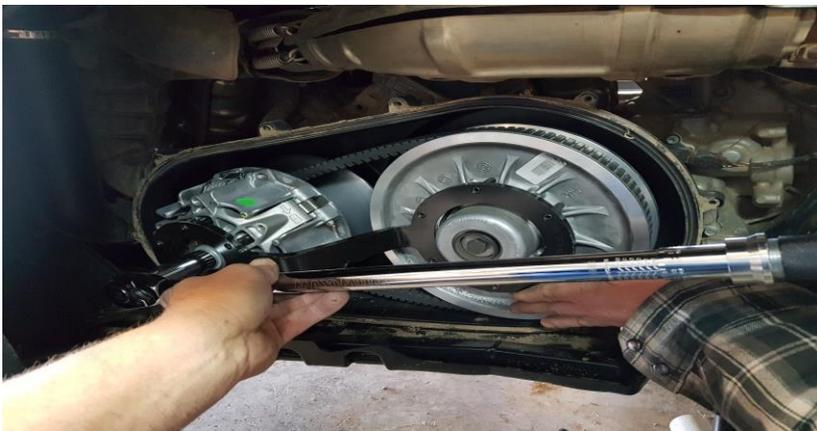
**Before installing belt make sure all sheave surfaces are clean and dry using non residue cleaner (Brake Cleaner) on a clean rag first then wipe.**
