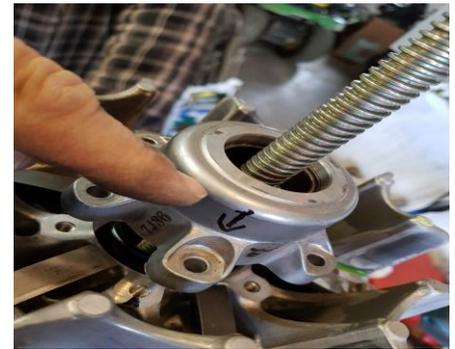
8) After removing the bolts, use the compressor tool to let pressure off the primary spring retainer cap. Install the new primary spring. Using the compression tool, carefully compress the new spring. Be careful when it gets close to seated that the rim edge is in proper position to seat correctly. It should go into place easily. Use blue removable thread locker on the threads of the bolts for the spring retainer cap. Torque primary spring cap screws to **(89 inch/lbs)** or 10 N.m
