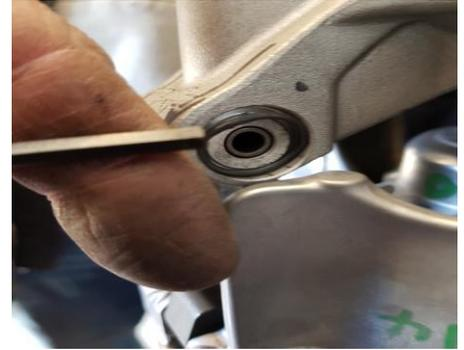
temporarily fold the flyweight lever arms to be out of the way for removal of the primary spring.
