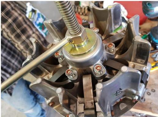
6) Mark the spring retainer cup and the clutch sheave surface with a marker for re-alignment later.
