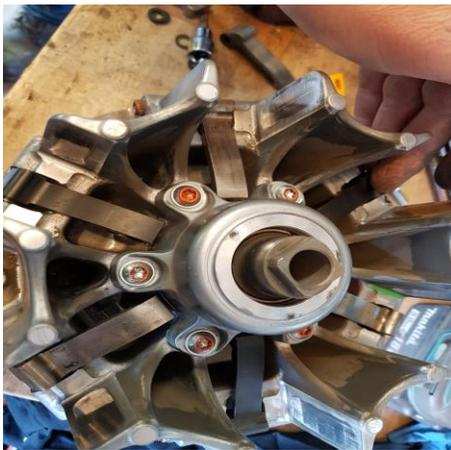
The 3 stock and 3 adjustable weights are alternating. The 3 stock are 120 degrees apart, as are the 3 new ones. – Every second one is replaced. THIS IS THE ONLY CONFIGURATION THAT 3 WEIGHTS CAN BE REPLACED.
