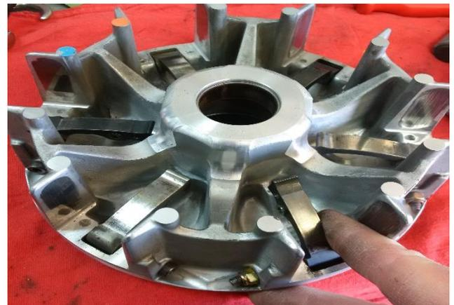
D) After setting up the provided flyweights **properly for your application** (\* See attached “flyweight set – up” for recommended application), install the new flyweights into the clutch and secure the pins / nuts the same way as they were removed. Be certain to put metal washers back in place (one each side of flyweight) before putting the pin through the weight.
