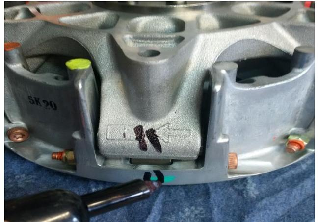
C) **VERY IMPORTANT:** CAN-AM ATV drive clutch has places for 6 flyweights. On this Outlander model all 6 positions are filled, and as many of you know (CAN AM service techs), there are other Can Am models with only 3 or 4 of the positions filled and some are not used at all. Example: Outlander 400 has only 4 flyweights.... With 2 of the 6 positions empty (180 degrees opposite each other). Some models only use 3 positions.
