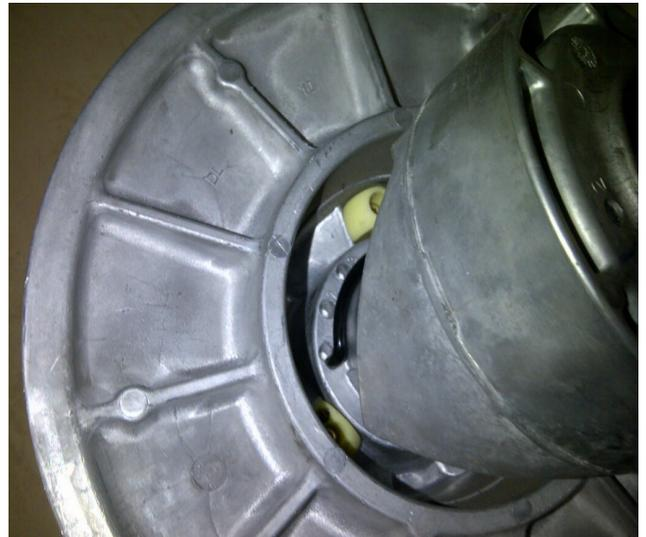
*Picture shows #1 hole in clutch*
