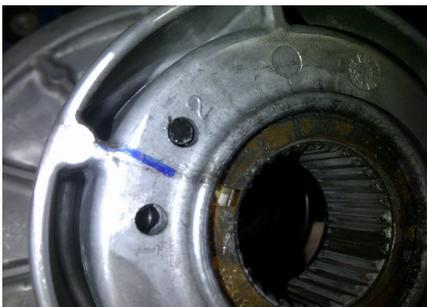
For this application, the secondary clutch spring will be remaining at **the factory setting of 2-2** in the torsional spring hook positions. (#2 hole in helix and #2 hole down in the clutch).
