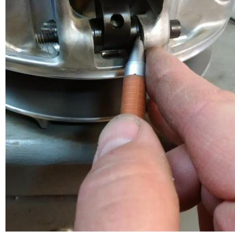
6) Install new primary spring into the clutch and re-install the cover onto the drive clutch (primary motor clutch). **Note: alignment marks.**
