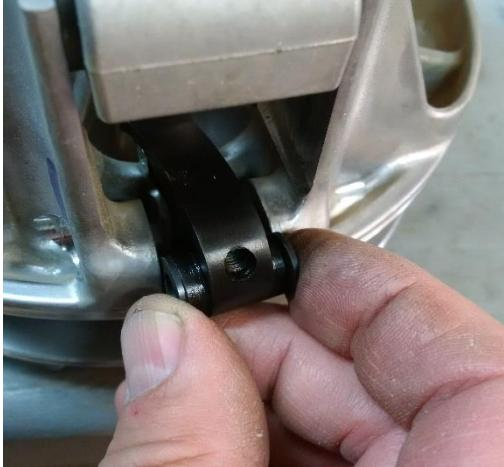
With stock clutches it is common to see the side of the clutch wearing from the flyweight pivot end gouging into the aluminum, even with only low miles. These thrust washers offer smooth function and prevent further wear.
