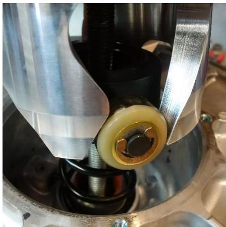
**Important!** – Be sure to have the “X” on the helix aligned with the x on the clutch.
